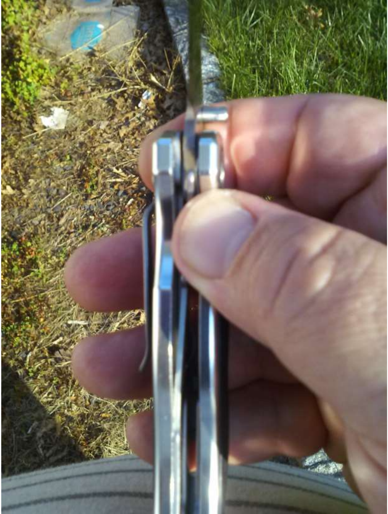
Photo 5 shows the thumb pushing the liner lock all the way to the left.
